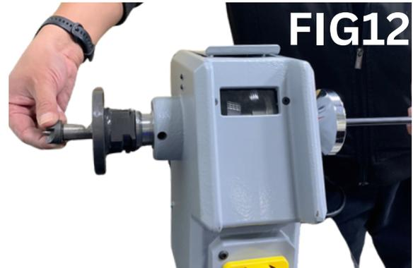
2. To re-insert the drive center, place it in the hole in the faceplate, and while using a block of wood and a hammer, tap the drive center to “set” it in the headstock.
